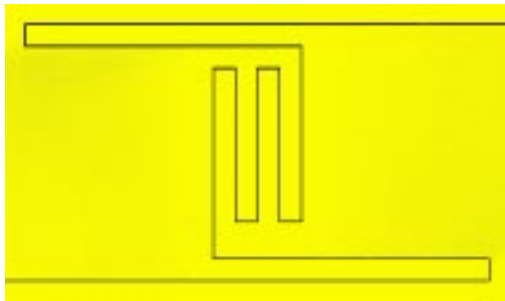
FIGURE 4. BASIC EXAMPLE OF A "GAP" TEST STRUCTURE LAYOUT. LARGE METAL AREAS ARE FOR SUBSEQUENT BOND PAD CONNECTIONS. GAP IS THE UNIFORM DARK LINE AT THE SPACING OF INTEREST.
