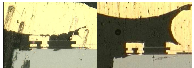
Figure 2. Cross Section of Bonded Wire Contacting Zipper (Left) and Sitting Above the Zipper (Right)
