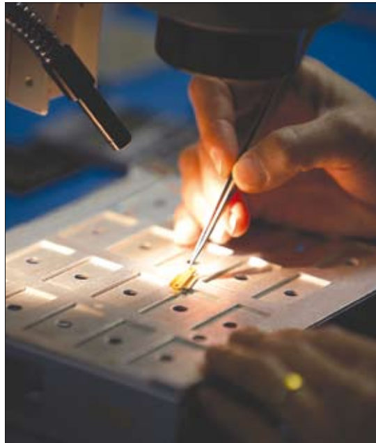
A technician in TriQuint's Boulder, CO, Design Center inspects lead coplanarity of a prototype PowerBand device.
