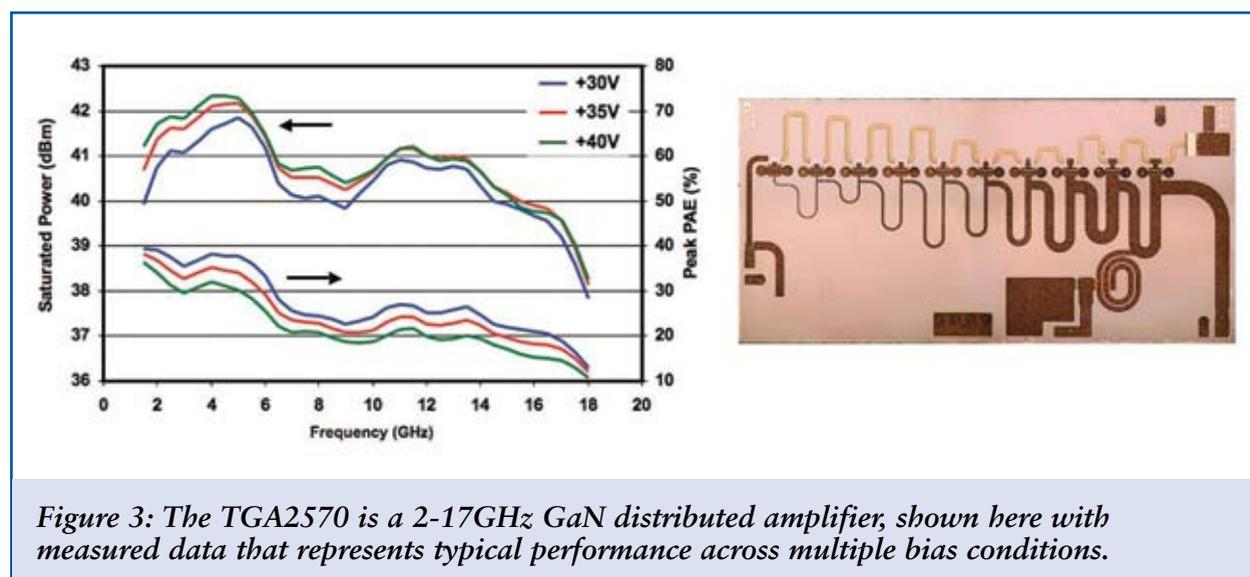
Figure 3: The TGA2570 is a 2-17GHz GaN distributed amplifier, shown here with measured data that represents typical performance across multiple bias conditions.
