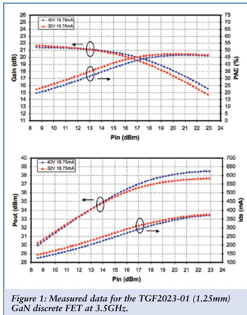
Figure 1: Measured data for the TGF2023-01 (1.25mm) GaN discrete FET at 3.5GHz.
