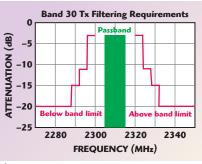
🔺 Fig. 4 Band 30 uplink filter requirements.
