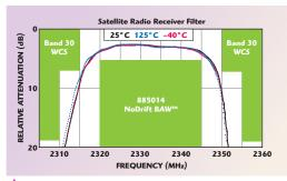
▲ Fig. 5 Performance of NoDrift<sup>™</sup> BAW satellite radio service filter over temperature range.
